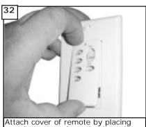
Attach cover of remote by placing over buttons and snaping into place.
